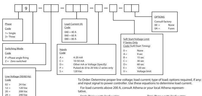
Single-Phase = <u>watts (load)</u> = amps Load Current volts (line) Three-Phase =  $\frac{\text{watts (load)}}{\text{Load Current } 1.73 \times \text{volts (line)}}$
