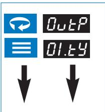
The first parameter that needs to be set in the Output Menu is the **Output Type**. There are three possible **Output Type** configurations: PID, On/Off, or Off. (If you are not sure which **Output Type** is best for your particular application, refer to the Glossary for an explanation of **Output Types**.) The remaining menu parameters in the Output Menu will change, depending on the **Output Type** selected.
