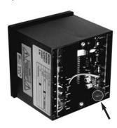
Figure 6. Location of Calibration Jumper.
