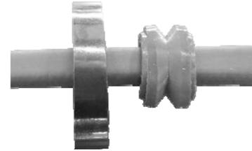
2. Carefully, lightly score/cut the outer jacket 3/4" (19 mm).
