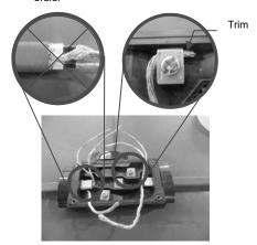
Install Gaskets and Covers onto the main box and secure covers with the screws.
