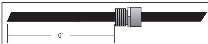
2. Assemble the connector and tighten, leaving six inches of cable extending through the connector.
