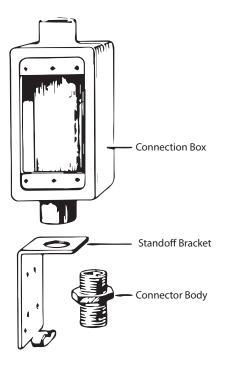
3. Guide the cold leads, braid and heater through the connector body into the box, insert the grommet in the connector body and tighten the connector cap. This should position the heating portion of the heater in the connector and the heater to cold lead connections about 2" out of the connector so that the heating portion will not enter the connection box.
