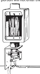
5. Connect the cold lead wires to power supply wires using approved wire connectors. Attach the braid pigtail to ground using the ring tongue terminal provided. Install the box cover.
