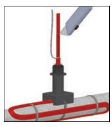
**5.** Score the inner insulation 6 inches from the end. Lightly cut the inner jacket up the center to end of heating cable and remove the inner jacket from the cable.
