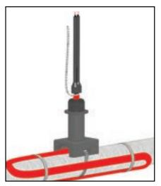
Strip each bus wire so that no black matrix material shows above the end of the rubber boot. Trim lead ends as needed.
